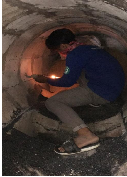
Loading of rice hull fuel (left) and igniting the rice hull inside the furnace burning chamber (right).
