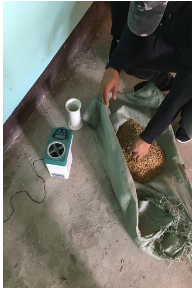
Moisture content of sampling material was tested every hour for moisture reduction monitoring.
