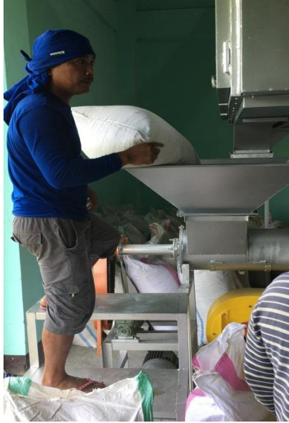
Loading of rice hull fuel (left) and igniting the rice hull inside the furnace burning chamber (right).
