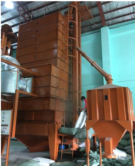
Loading of sampling materials to the 6 tonners (left) and 12 tonners (right) recirculating mechanical dryer.
