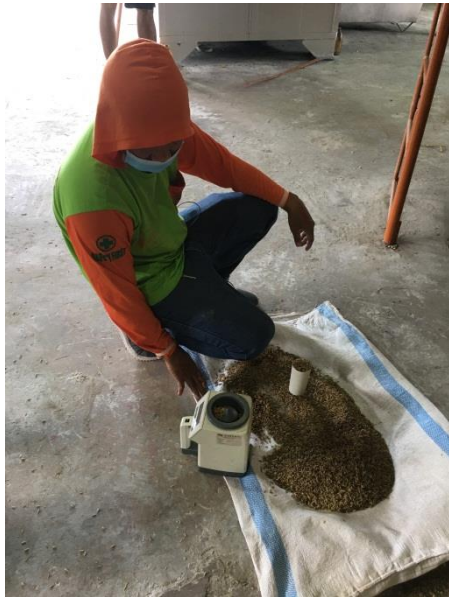
Testing of moisture content of sample (left) and measuring the current use of the dryer (right).
