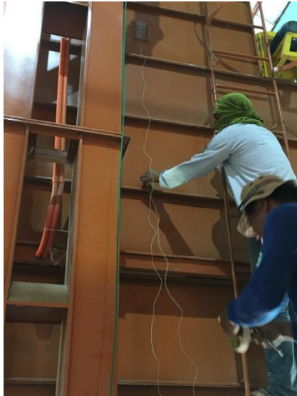
Positioning of thermocouples in the drying chamber (left) and plastic tube in the plenum chamber (right).
