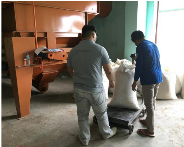
Weighing all the rice hull fuel to be use in the testing (left) and initial firing of rice hull fuel in the burning chamber of the furnace (right).
