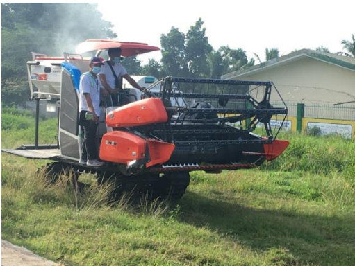
Operators actual operation of the rice combine harvester (left) and parts maintenance and adjustments of the cutting mechanism (right).
